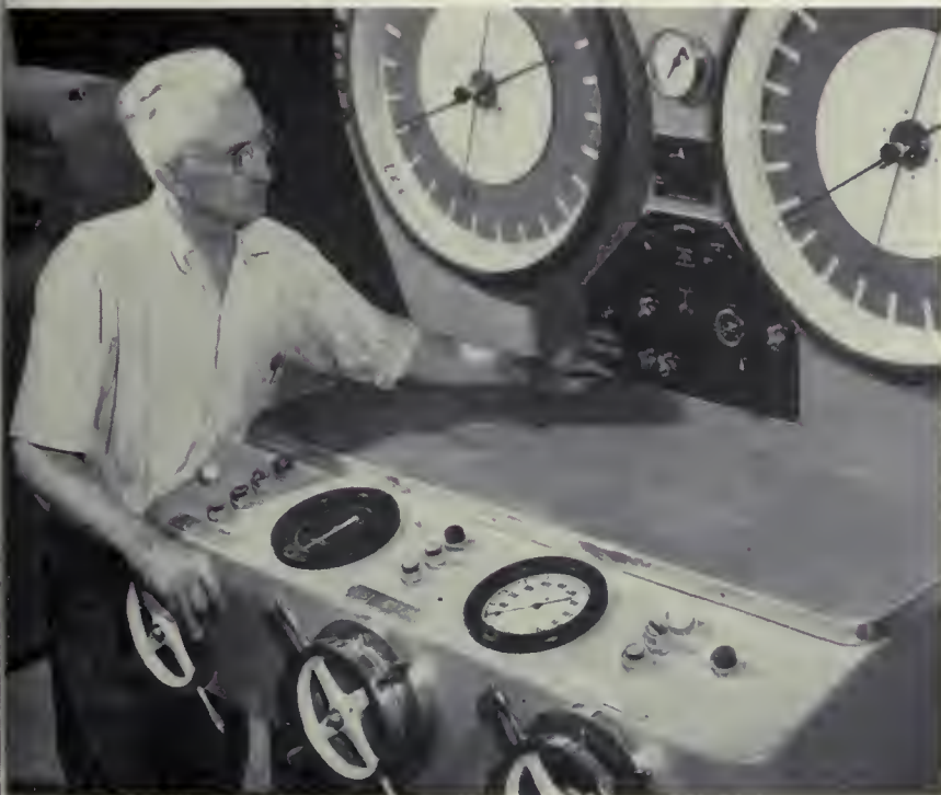
NEVER MISSES A DAY'S WORK. —Earl D. Newton at the control panel of the five-million-pound capacity universal testing machine in Denver's Reclamation Engineering Center. Photo by Charles Knell, Region 6 photographer.
